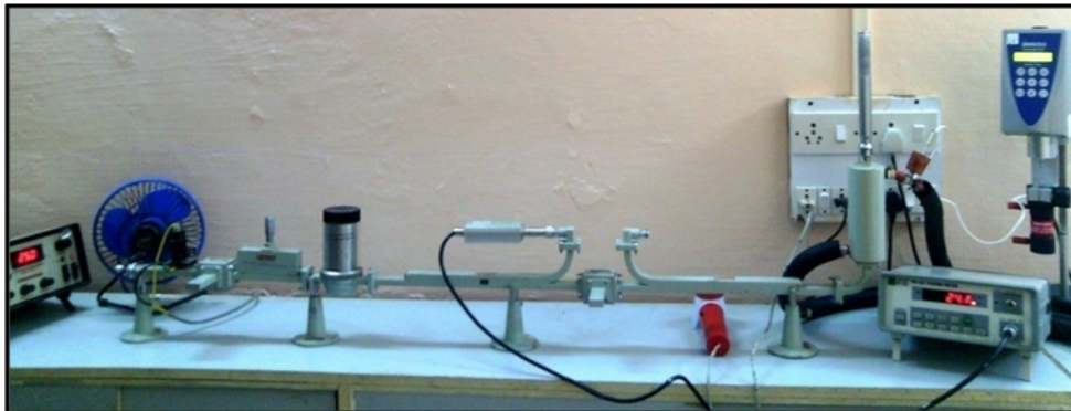
Fig. 1: The Experimental setup of X-band Microwave Bench
